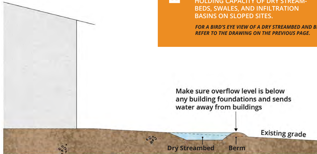
DRY STREAMBED BERM DETAIL FOR SLOPED SITES
