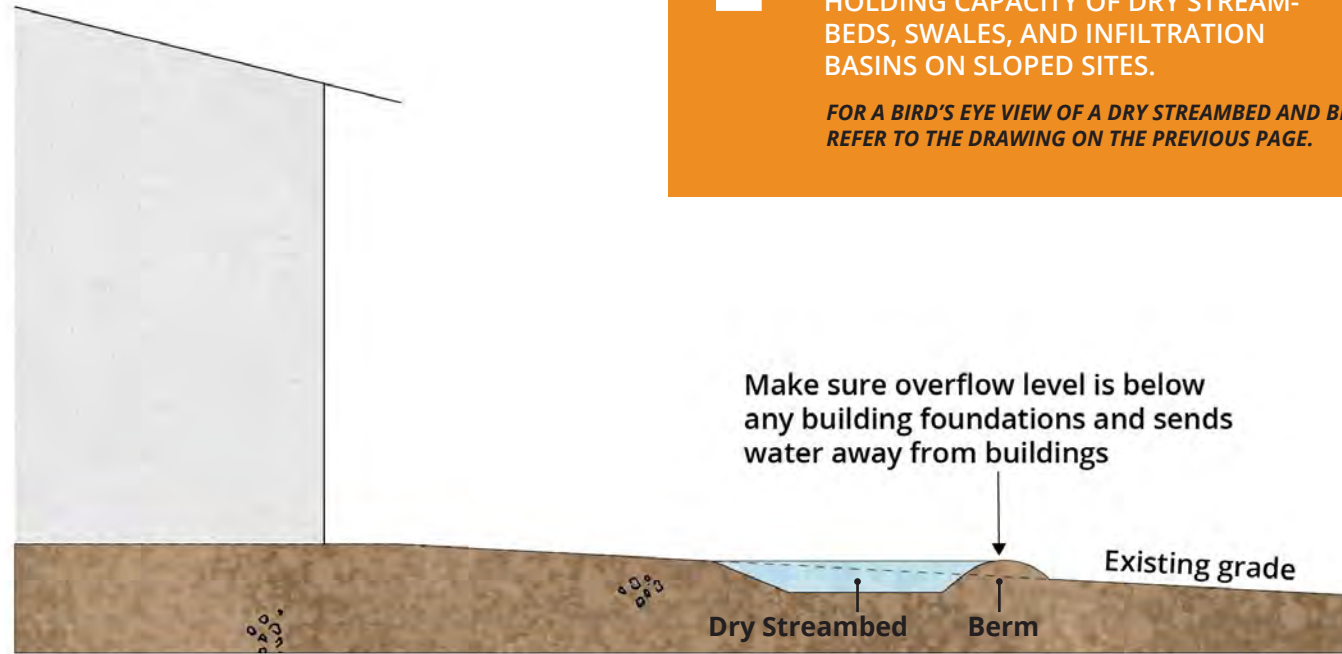
DRY STREAMBED BERM DETAIL FOR SLOPED SITES
